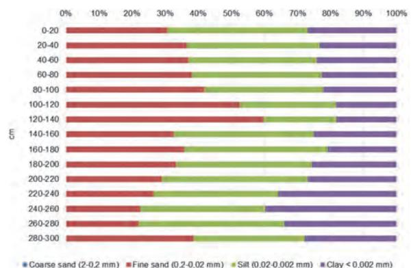
Fig. 3. Distribution of granulometric composition in the case of soil samples originating from the BA5 monitoring well; source: own elaboration
