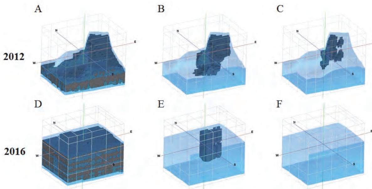
Fig. 7. Spatial distribution of NH<sub>4</sub><sup>+</sup> concentrations down to the depth of 3 m from the surface; A, D: higher than 0.5 mg·dm<sup>-3</sup>, B, E: higher than 30 mg·dm<sup>-3</sup>, C, F: the extension of the water body with an NH<sub>4</sub><sup>+</sup> concentration higher than 90 mg·dm<sup>-3</sup>; source: own elaboration
