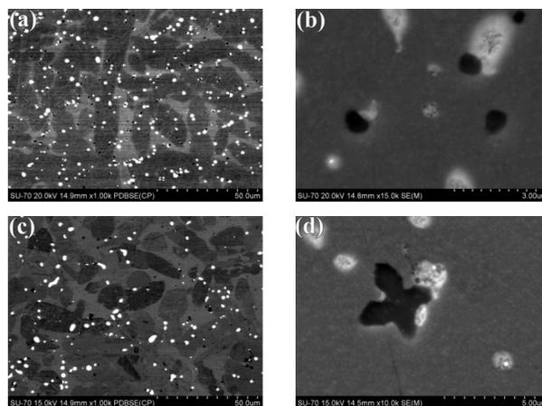
Fig. 2. The microstructure of MO59 alloy - the feed structure I (a, b) and the feed structure II (c, d) observed by means of scanning electron microscopy (SEM)
