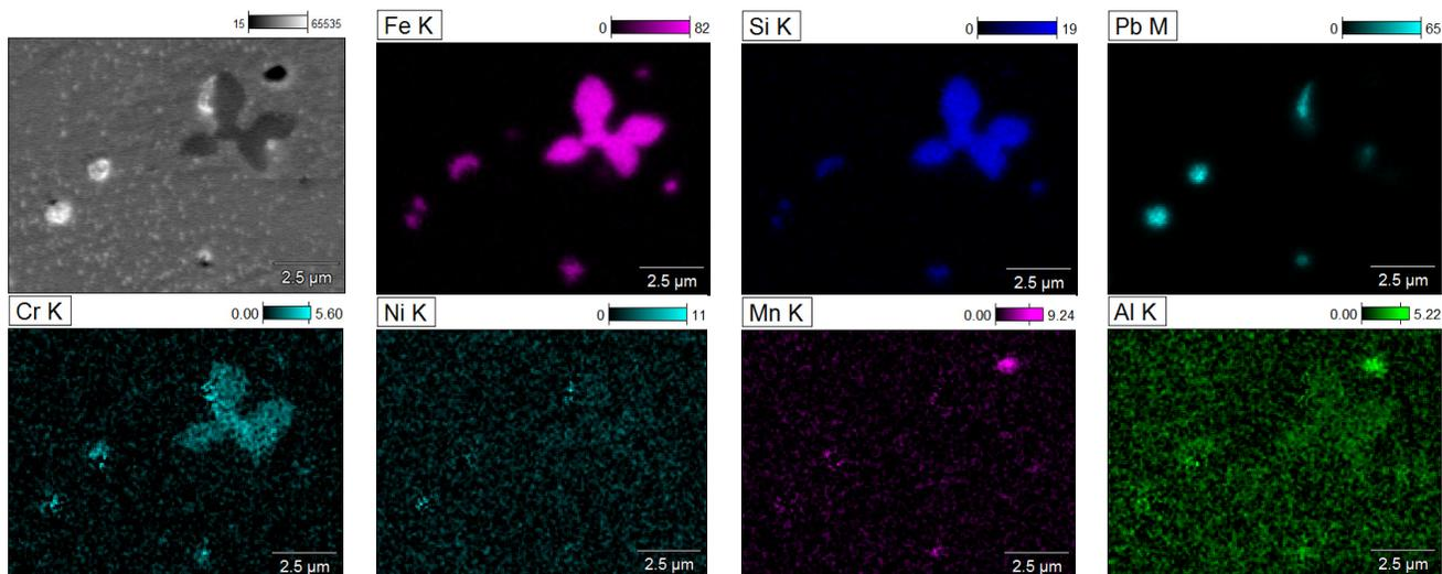
Fig 4. Element map distribution of different elements received for MO59 alloy - the feed structure II (SEM mapping). Results are in atomic %
