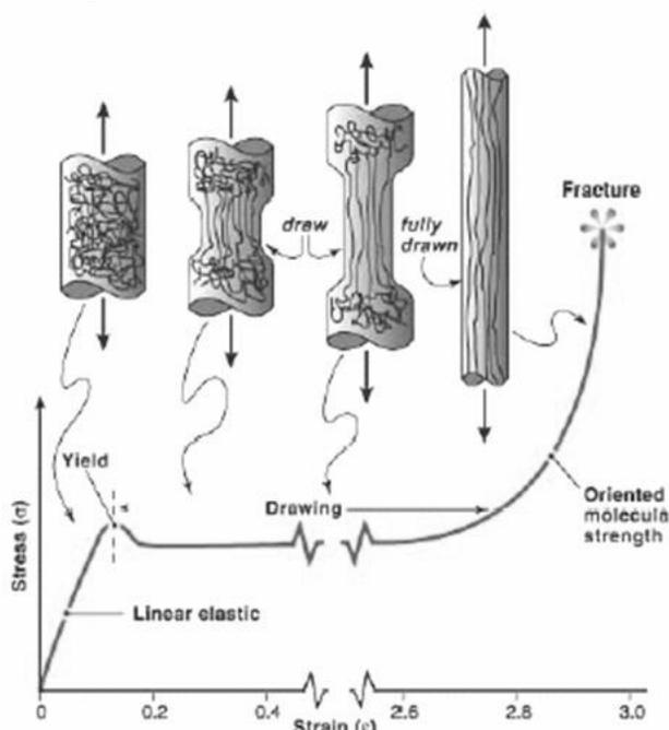
Fig. 1. Stress-strain curve and elongation of polymer chains during deformation [7].
