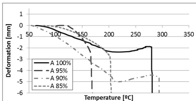
Fig. 8. Hot distortion research of moulding sand mixtures with different content of alkyd resin
