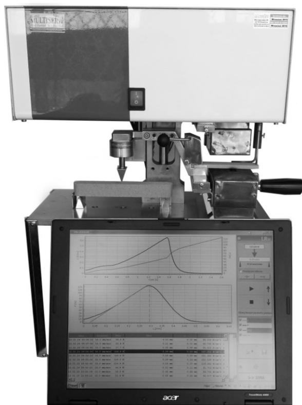
Fig. 2. New prototype testing appliance LRu-DMA produced by MULTISERW-Morek company.
