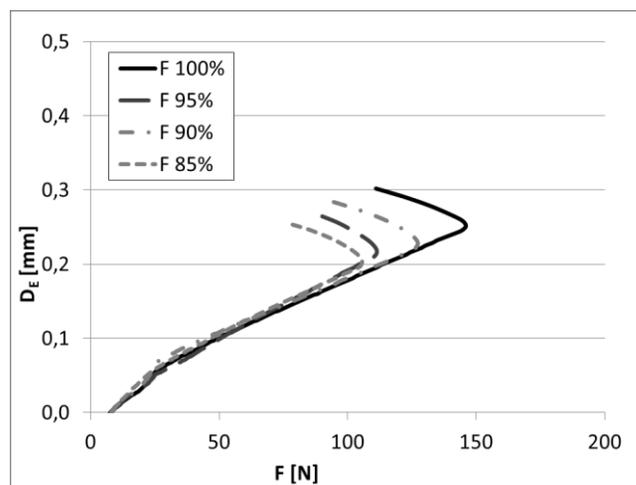
Fig. 3. Elasticity of moulding sand mixtures with different content of furfuryl resin
