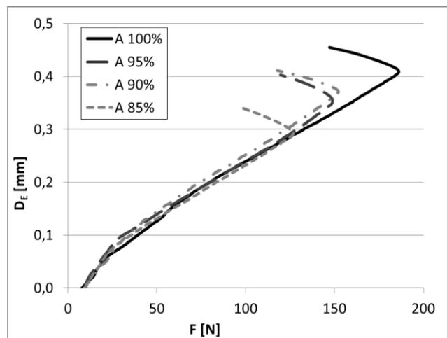
Fig. 5. Elasticity of moulding sand mixtures with different content of alkyd resin
