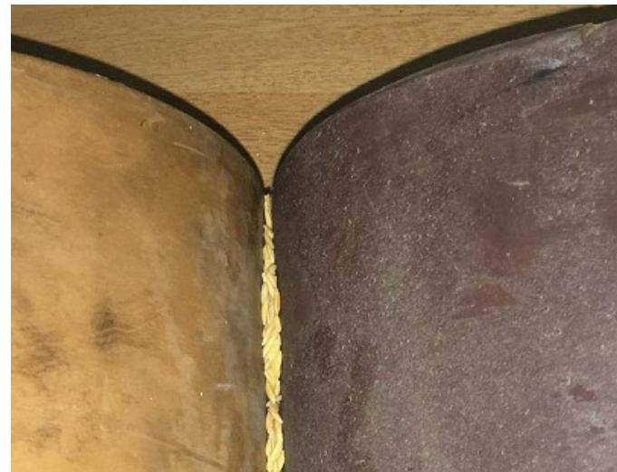
Fig. 2. Photograph of paddy in between rubber rollers before husk removal
