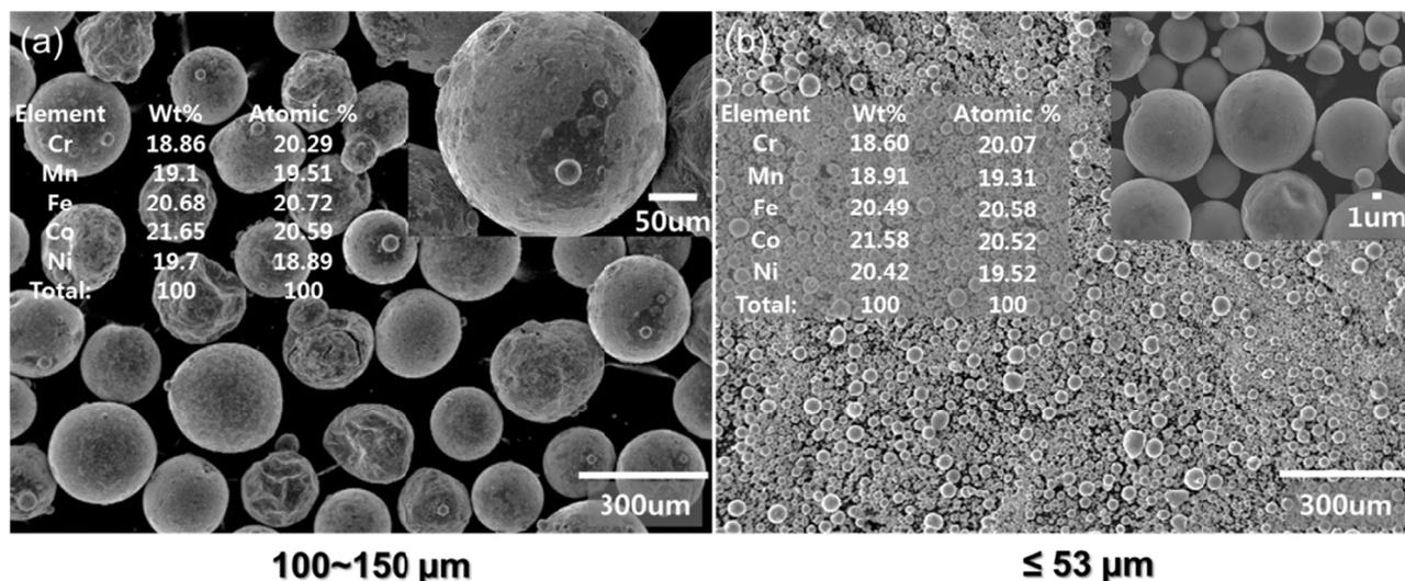
Fig. 2. Microstructure and surface elemental analysis of atomized HEA powder (a) 100~150  $\mu\text{m}$  large sized powders, (b) <53  $\mu\text{m}$  small sized powder
