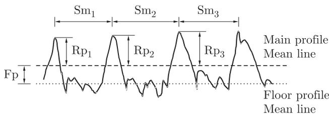
Fig. 6. Representation of roughness structures in terms of the new roughness parameters: Maximum Profile Peak Height ( $R_p$ ), Mean spacing of profile irregularities ( $R_{Sm}$ ), and Floor Distance to Mean Line ( $F_p$ ), Kandlikar et al. (after Ref. 38)
