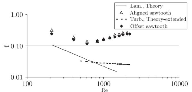
Fig. 4. Fully developed friction factor vs. Reynolds number, both based on hydraulic diameter; water flow.  $D_h = 953 \mu\text{m}$ , height = 500  $\mu\text{m}$ , width = 10.03 mm,  $\epsilon/D_h = 0.0735$ , Kandlikar et al. (after Ref. 38)
