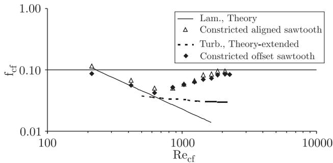
Fig. 5. Fully developed friction factor vs. Reynolds number, both based on constricted flow hydraulic diameter; water flow. Hydraulic diameter based on constricted flow,  $D_{h,cf} = 684 \mu\text{m}$ , channel height at saw-tooth base =  $500 \mu\text{m}$ , constricted height =  $354 \mu\text{m}$ , channel width =  $10.03 \text{ mm}$ ,  $\varepsilon/D_{h,cf} = 0.1108$ , Kandlikar et al. (after Ref. 38)
