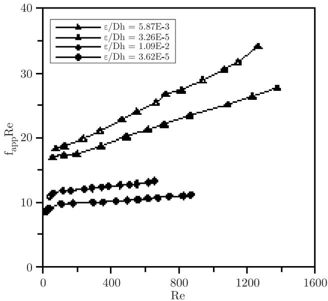
Fig. 2. Comparison of  $f_{app} Re$  product versus  $Re$  plots for two sets of microchannels with different relative roughness surfaces, Wu and Cheng (after Ref. 35)
