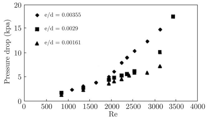
Fig. 1. Plot of pressure drop versus Re for different relative roughnesses with water flow in a 0.62 mm diameter tube, Kandlikar et al. (after Ref. 34)
