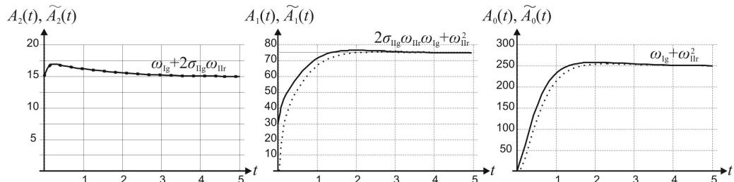
Fig. 14. Results of reducing the cascade section connection – waveforms of substitute system parameters (variant A – solid line, variant B – dot line)
