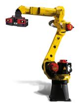
Fig. 2. Industrial robot with optical measuring system GOM Atos Triple Scan
