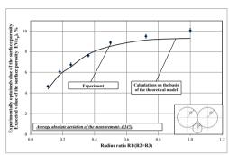
Fig. 4. Comparison of the expected value of the surface porosity  $EV(\epsilon_p)$  and its value obtained experimentally  $(\epsilon_{p \text{ (exp)}})$ . Grains system:  $R_1$ =0.065 mm;  $R_2$ = $R_3$ = var; quantitative participation of components: n = k = 1 = 33.33%.
