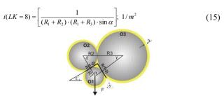
Fig. 3. Model system for calculating the surface area of bonding grains of various sizes in the system corresponding to the coordination number, LK=8
