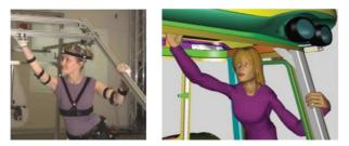
Fig. 7. Virtual reality in assembly process analysis lets verify the reachability to improve the design of product [18].
