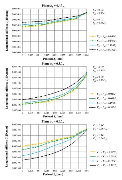
Fig. 9. Longitudinal stiffness  $C_x$  for the assumed variation of load
