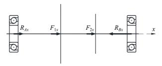
Fig. 3. Calculation scheme for axial reactions of supports
