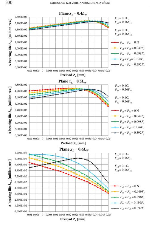
Fig. 6. Fatigue life of bearing A
