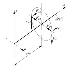
Fig. 5. Assumed variations of loads of the bearings
