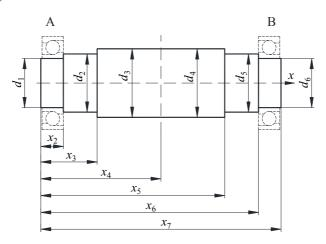
Fig. 4. Draft of a model shaft
