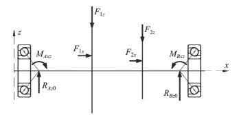
Fig. 2. Calculation scheme for transverse reactions of supports
