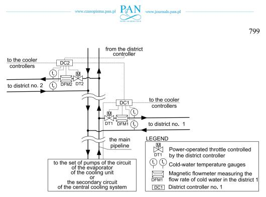
Fig. 3. A control system for regulating the flow of cold water into districts of a cooling system
