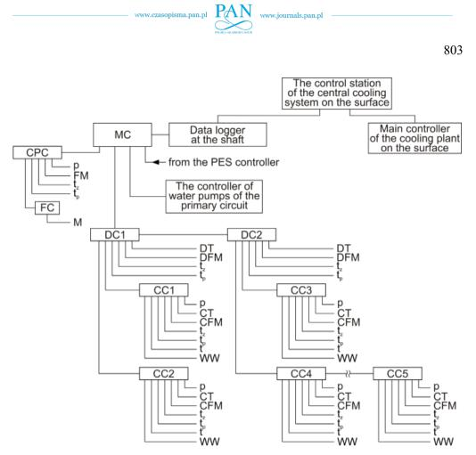
Fig. 7. Structure flowchart of the systems for the monitoring and control of the parameters of cold water in a central cooling system
