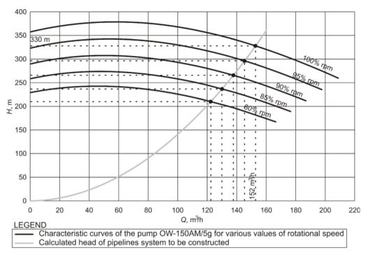
Fig. 2. Modifying the working parameters of a pump with the designation OW-150AM/5g by adjusting the rotational speed of the rotor in a sample central cooling system
