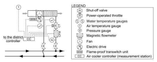
Fig. 5. Conection diagram of an air cooler controller with measuring devices and actuators
