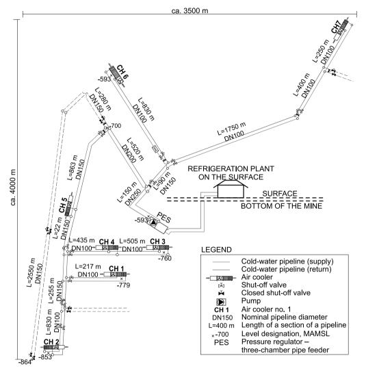
Fig. 1. Layout of a secondary circuit of a exemplary central cooling system
