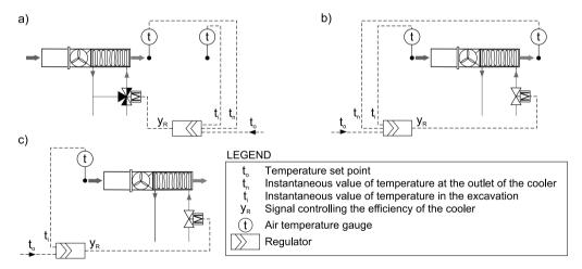
Fig. 4. Regulating the cooling capacity of an air cooler, a) a cascade control system (self- and relay-operated regulators) with regulators in one package, b) a cascade control system with a packed regulators and air temperature measured in the excavation in front of the cooler, c) a self-operated control system for regulating air temperature in the excavation in front of the cooler
