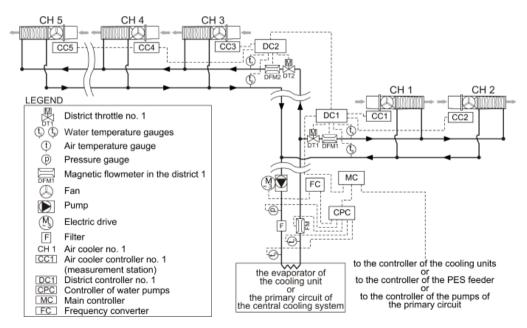
Fig. 6. Schematic diagram of the systems for the monitoring and control of the parameters of cold water in a central cooling system
