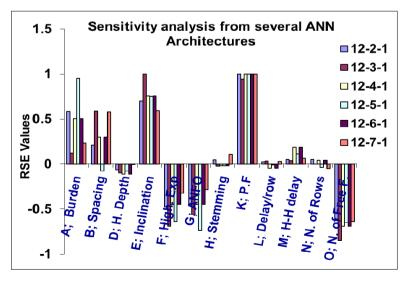
Fig. 4. Relative strength effects (RSEs) of variables on backbreak
