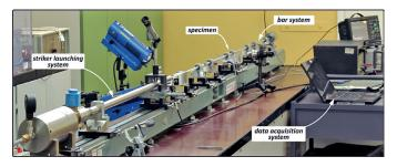
Fig. 1. View of the arrangement used for classical split Hopkinson compression bar
