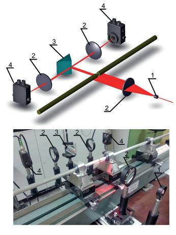
Fig. 3. The scheme of the laser extensioneter and the arrangement; 1 – Powell lens, 2 – plano-convex spherical lens, 3 – knife edge right angle prism mirror, 4 – detectors
