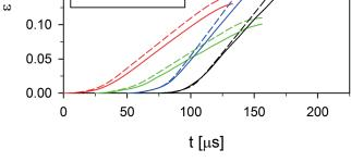
Fig. 6. Comparison of strain history in the specimens obtained from strain gage (dashed lines) and laser extensometer measurments (solid lines): a) Al 5251, b) Cu OFE. The lines were shifted in the increment of 25 ms for ease of comparison
