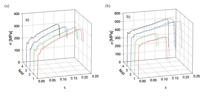
Fig. 7. The engineering compression stress-strain curves from strain gage (dashed lines) and laser extensometer measurments (solid lines) of: a) Al 5251, b) Cu OFE
