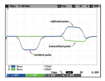
Fig. 2. The raw waves signals measured by the strain gages for aluminum specimen
