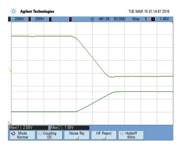
Fig. 4. Raw waves signals measured by the laser extensioneter, input bar, brown – Detector 1, output bar, green – Detector 2
