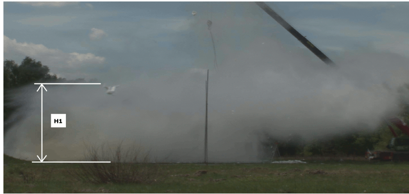
Fig. 1. Determination of the upper edge of the water-spray cloud with respect to a fixed reference level. The initial stage of cloud's fall is registered.
