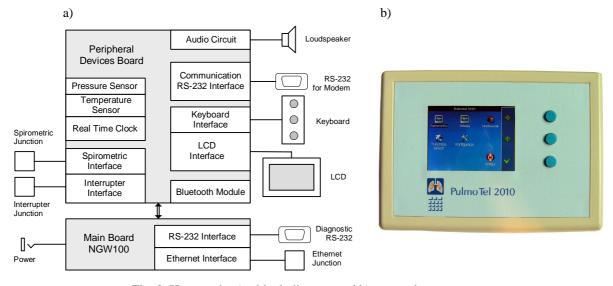
Fig. 2. Home unit: a) a block diagram and b) outward appearance.
