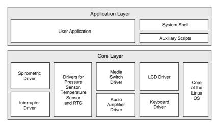
Fig. 3. Block diagram of home unit's firmware.
