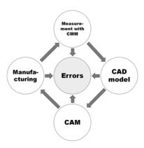
Fig. 10. The sources of surface reconstruction errors.
