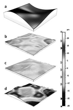
Fig. 8. Reconstruction errors [ $\mu$ m]: a 3D surface profile (a); the values of x component of the error ( $\delta_x$ ) (b); the values of y component of the error ( $\delta_y$ ) (c); the values of z component of the error ( $\delta_z$ ) (d).
