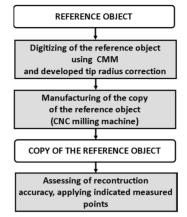
Fig. 1. A workflow of the proposed procedure.
