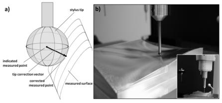
Fig. 2. The idea of coordinate measurement; the principle of probe tip radius correction (a); measurement by means of CMM (b).
