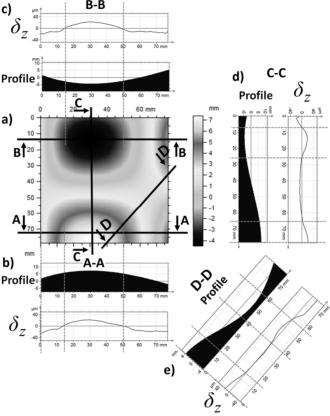
Fig. 9. The values of  $\delta_z$  error components for respective surface profiles; the reference object (a); the profile and  $\delta_z$  error components for the cross-sections: (A-A), (B-B), (C-C), (D-D).
