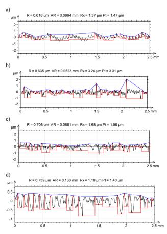
Fig. 8. Examples of the motif graphs for hard turned (a); ground with Al<sub>2</sub>O<sub>3</sub> wheel (b); ground with CBN wheel (c) and honed (d) surfaces.
