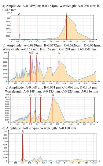
Fig. 11. The averaged power spectral density for turned (a); ground with Al<sub>2</sub>O<sub>3</sub> wheel (b); ground with CBN wheel (c) and honed (d) surfaces.
