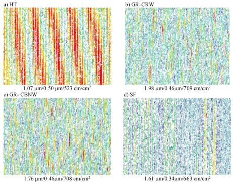
Fig. 4. Vectorised micro-valley networks for turned (a); ground with Al<sub>2</sub>O<sub>3</sub> wheel (b); ground with CBN wheel (c) and honed (d) surfaces. Three values give the average depth, width and density of micro-valleys.
