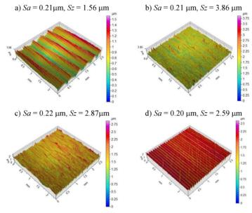
Fig. 1. Surface textures produced by HT (a); ground using Al<sub>2</sub>O<sub>3</sub> (b); CBN wheel (c) and honed (d).
