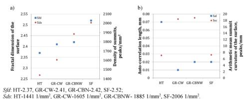
Fig. 10. Functional relationships between selected 3D S-parameters and the fractal dimension.
