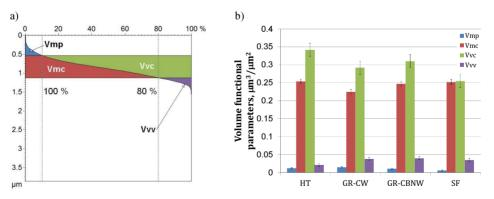
Fig. 5. Functional volumetric parameters for different finishing operations: distribution of volume parameters for hard turning (a); distributions for all machining operations (b).
