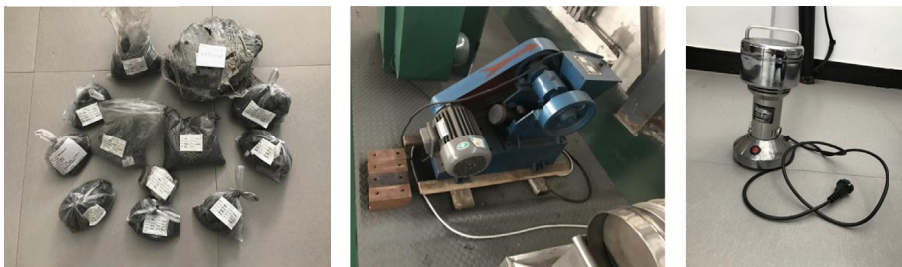
Fig. 1. The coal specimens and corresponding crushing device
