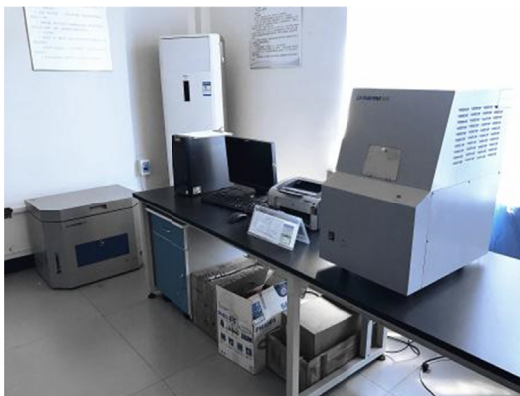
Fig. 5. Two-furnace automatic coal proximate analyzer
