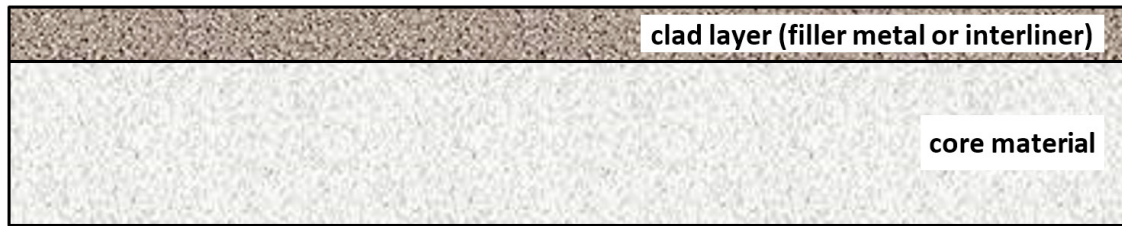
Fig. 1. An example of the structure of the material used in manufacture of aluminum heat exchangers
