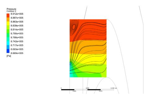
Figure 23: Pressure and streamlines in radial cross-section of inlet spiral, variant 6.
