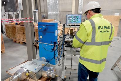
Fig. 7 VNA test and installation of 26,352 MHz circulators
