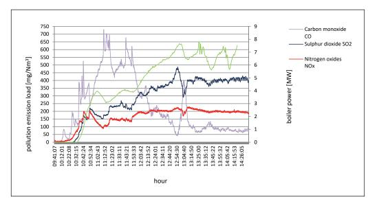
**Fig. 4.** Pollutant concentrations in the exhaust gases during boiler no. 1 start-up in Heating Plant A – compounds: CO, SO<sub>2</sub> and NO<sub>x</sub>
