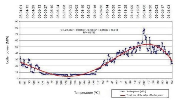
Fig. 2. Changes of boiler heating power vs. outdoor temperature in the period of one selected year for Heating Plant A (Różycka-Wrońska, 2016)
