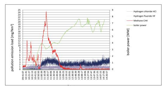
Fig. 6. Pollutant concentrations in the exhaust gases during boiler no. 1 start-up in Heating Plant A – compounds: hydrogen chloride, hydrogen fluoride, methane
