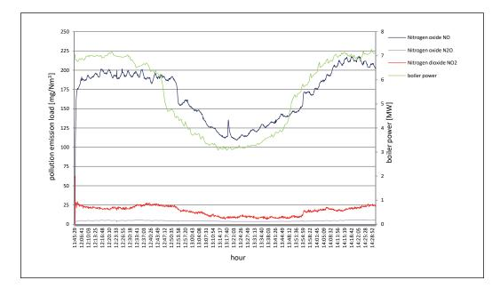
**Fig. 8.** Pollutant concentrations in the exhaust gases during power changes of boiler no. 2 in Heating Plant A – nitrogen compounds: N<sub>2</sub>O, NO and NO<sub>2</sub>
