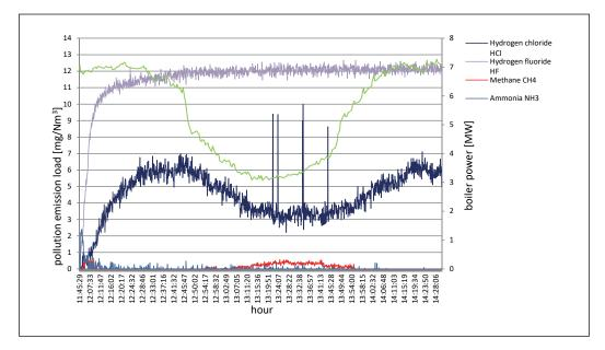
Fig. 9. Pollutant concentrations in the exhaust gases during power changes of boiler no. 2 in Heating Plant A - compounds: hydrogen chlorine, hydrogen fluoride, methane, ammonia
