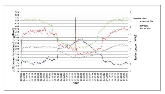
**Fig. 7.** Pollutant concentrations in the exhaust gases during power changes of boiler no. 2 in Heating Plant A – compounds: CO, SO<sub>2</sub> and NO<sub>x</sub>
