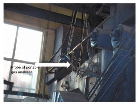
Fig. 3. Location of the gas analyser probe during experimental measurements of the concentration of pollutants in the exhaust gases
