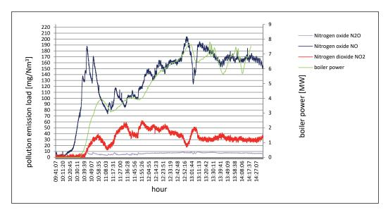
**Fig. 5.** Pollutant concentrations in the exhaust gases during boiler no. 1 start-up in Heating Plant A – nitrogen compounds: N<sub>2</sub>O, NO and NO<sub>2</sub>
