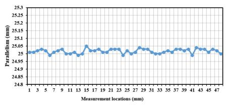
Fig. 6. Measured thickness variation for estimation of parallelism in the RSB.
