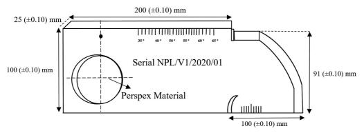
Fig. 1. Ultrasonic IIW V1 RSB (side view), used for the functional validation of UPE devices.
