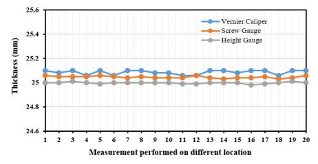
Fig. 2. Thickness measurement variation of the RSB by using the Vernier caliper, screw gauge, and height gauge.
