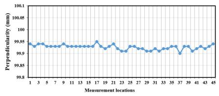
Fig. 7. Measured thickness variations for estimation of perpendicularity in the RSB.
