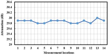
Fig. 5. Measured ultrasonic attenuation in the RSB.
