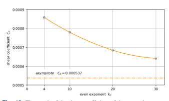
**Fig. 10.** The graph of the shear coefficient of the exemplary square sandwich plate  $(e_0 = 1/20)$
