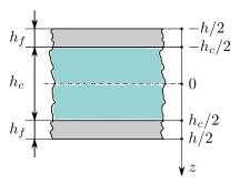
Fig. 2. Scheme of the structures of the sandwich cylindrical panel
