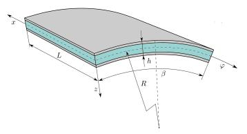
Fig. 1. Scheme of the sandwich cylindrical panel
