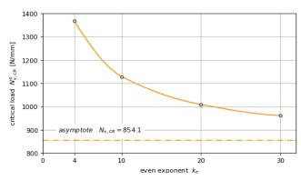
**Fig. 9.** The graph of the critical load of the exemplary square sandwich plate  $(e_0 = 1/20)$
