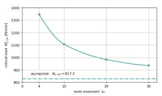
**Fig. 11.** The graph of the critical load the exemplary square sandwich plate  $(e_0 = 1/30)$
