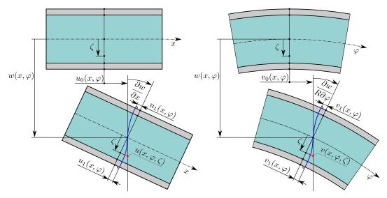
Fig. 4. Scheme of the deformation of the straightnormal line – the nonlinear hypothesis
