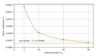
**Fig. 6.** The graph of the shear coefficient of the exemplary cylindrical sandwich panel ( $e_0 = 1/20$ )
