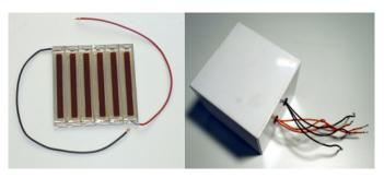
**Fig. 3.** View of the B2 photovoltaic dye module with a photosensitive field area of 33.6 cm<sup>2</sup> and a new supercapacitor with a capacitance of  $C_{SC} = 60$  F, rated operating voltage  $U_C = 3$  V and series resistance  $R_S = 106 \text{ m}\Omega$
