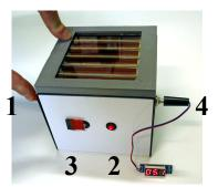
Fig. 6. A model of a constructed solar charger based on dye-based photovoltaic modules and new supercapacitors
