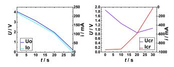
**Fig. 9.** Graphs of discharge of a model of a solar charger ( $C_{SC} = 60$  F)
