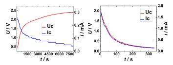
Fig. 5. Charge and discharge characteristics of a new supercapacitor  $(C_{SC} = 60 \text{ F})$
