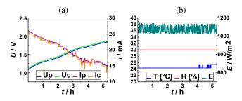
**Fig. 10.** (a) Graph of the boost of the solar charger model, (b) graph of the environmental conditions during the measurement of the boost of the solar charger model
