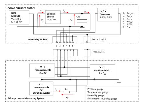
Fig. 7. Microprocessor stand for testing the parameters of functional models of solar chargers – block diagram
