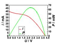
**Fig. 4.** Current-voltage characteristics of a dye module with a photosensitive field area of 33.6 cm<sup>2</sup> ( $V_{OC} = 3.8$  V,  $I_{SC} = 25.9$  mA,  $V_{max} = 1.6$  V,  $I_{max} = 12.2$  mA,  $P_{max} = 19.7$  mW,  $R_{so} = 207 \Omega$ ,  $R_{sho} = 96 \Omega$ ,  $\eta = 0.8\%$ , FF = 0.2)
