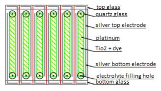
Fig. 1. Architecture of the DSSC module with dimensions of  $100 \times 100$  mm
