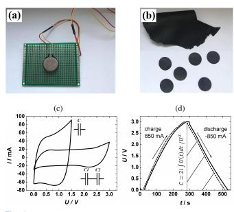
**Fig. 2.** (a) A supercapacitor in a CR2032 housing placed on a PCB in a pocket for diagnostic tests, (b) Supercapacitor electrodes cut from the YP-80F carbon sheet, (c) Voltammetric curves ( $v = 50 \text{ mV s}^{-1}$ ) of a supercapacitor (U = 1.5 V) and two serially connected supercapacitors (U = 3 V) within one coin housing, (d) Galvanostatic curve of complete modules (i = 850 mA)
