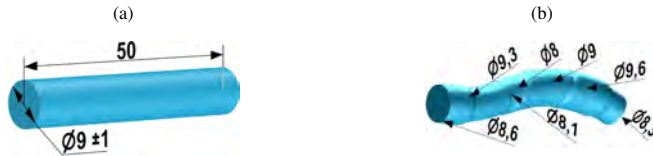
Fig. 17. (a) ISO specification for shaft diameter; (b) shaft that fulfills the specification. [authors' drawing]
