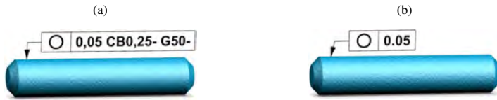
Fig. 19. Equivalent tolerance specifications. (a) Roundness tolerance (ISO); (b) circularity tolerance (ASME). [authors' drawing]
