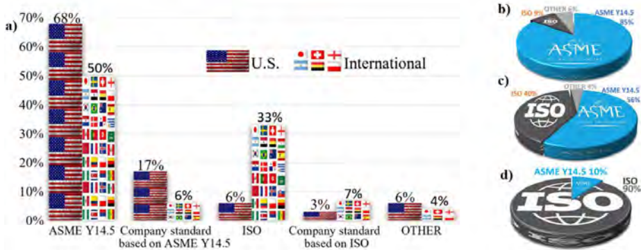
Fig. 1. (a) Percentage of drawings that use a specific standard in international and US companies; (b) use of standards in US companies; (c) use of standards in multinational companies; (d) use of standards in Polish companies [18].
