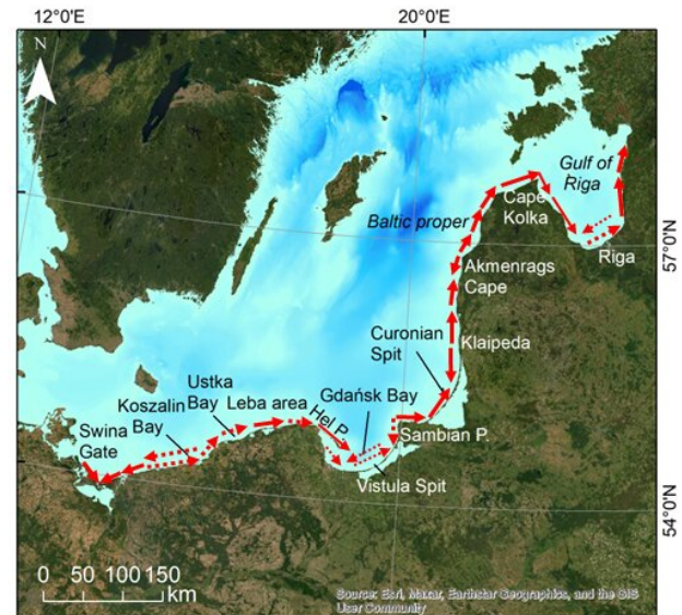
Figure 6. A generalised view of the long-term alongshore sediment transport pattern on the southern and eastern shores of the Baltic Sea. “Hel P.” is the Hel Peninsula and “Sambian P.” is the Sambian Peninsula. The dotted lines reflect variable-direction transport. See references to the sources used in Harff et al. (2017). Amended from Harff et al. (2017).
