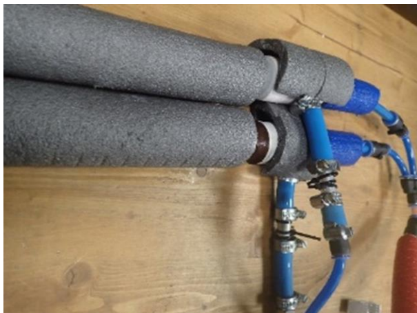
Fig. 5. Laboratory station for two internal heat exchangers (IHXs).
