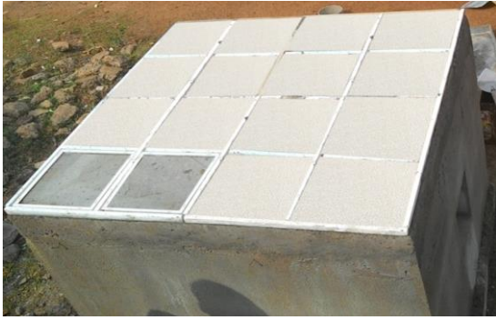
Fig. 2. Glass fibre roof slab model.
