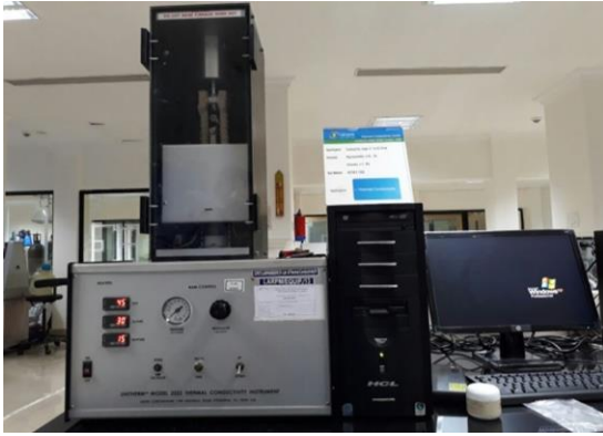
Fig. 10. Measurement of thermal conductivity according to ASTM E1530. Image courtesy: CIPET, Bhubaneswar.
