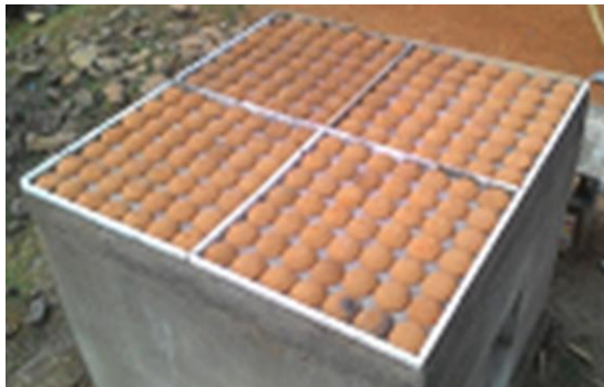
Fig. 3. Earthen pot roof slab model.
