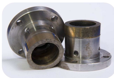
Fig. 4. Grinding tools for machining spherical elements
