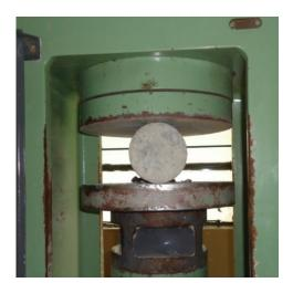
Fig. 7. Split tensile testing set up
