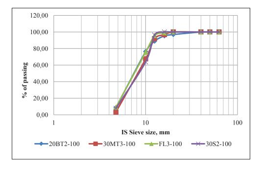
Fig. 8. Gradation of various types of aggregates
