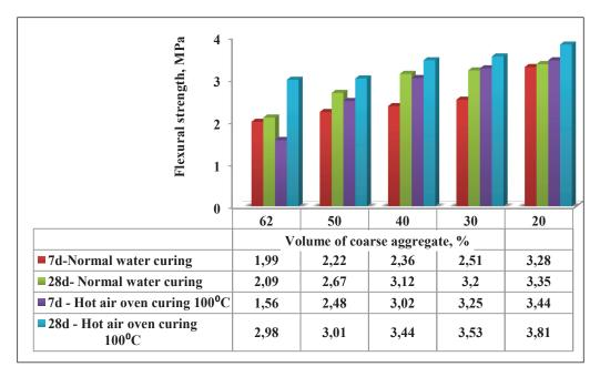
Fig. 18. Flexural strength of fly ash aggregate concrete in water curing and hot air oven curing
