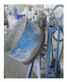
Fig. 1. Disc pelletizer machine
