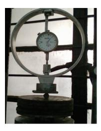
Fig. 3. CBR testing machine
