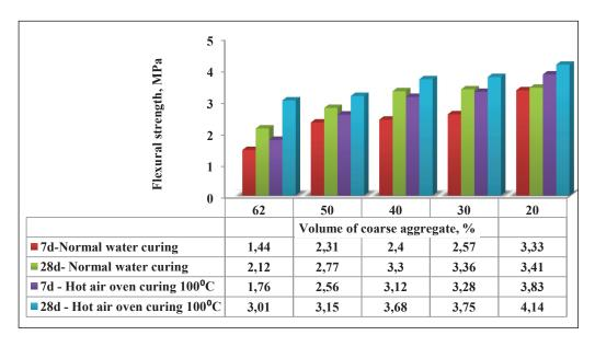
Fig. 21. Flexural strength of fly ash-metakaolin aggregate concrete in water curing and hot air oven curing
