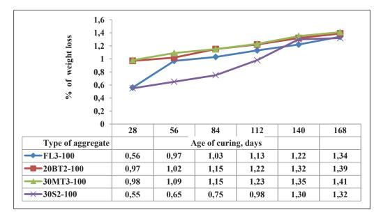
Fig. 12. Alternate wetting and drying process of light weight aggregate at different days of curing
