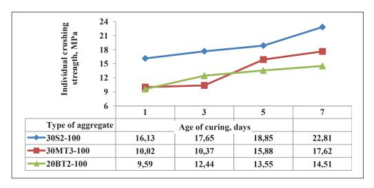
Fig. 10. Crushing strength of various types of fly ash aggregate at oven curing 100°C (10 mm diameter of pellet
