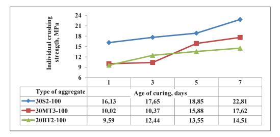
Fig. 11. Crushing strength of different types of fly ash aggregate at oven curing 100°C (12 mm diameter of pellets)
