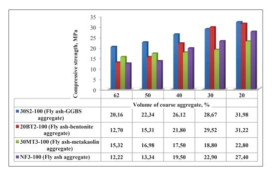
Fig. 15. Compressive strength of different types of fly ash aggregate concrete in Hot air oven curing at 100°C (28 days strength)
