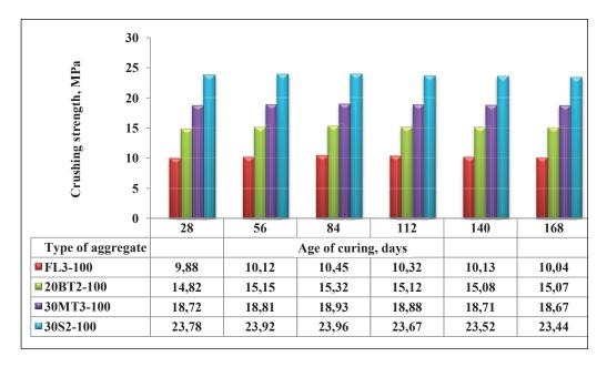
Fig. 13. Crushing strength of aggregates cured in alternate wetting and drying environment (10 mm diameter of pellets)
