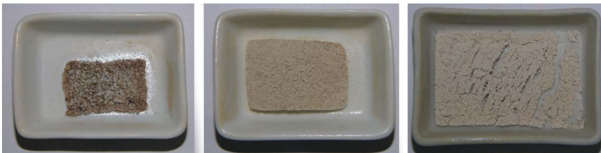
Fig. 8. Slag samples from olive cake heated in the muffle furnace at the temperature of 1000°C, from the left: without additive, with Bolesław Śmiały coal ash and Turów lignite I ash
