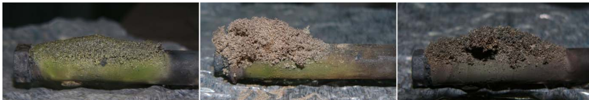
Fig. 10. Slag samples collected on the probe during biomass-firing, from the left: cereal straw, cereal straw with Turów lignite I ash and Bolesław Śmiały coal
