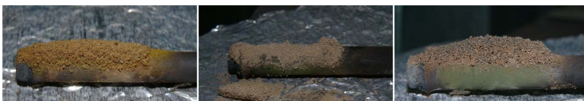
Fig. 11. Slag samples collected on the probe during biomass-firing, from the left: olive cake, olive cake with Turów lignite I ash and with Bolesław Śmiały coal
