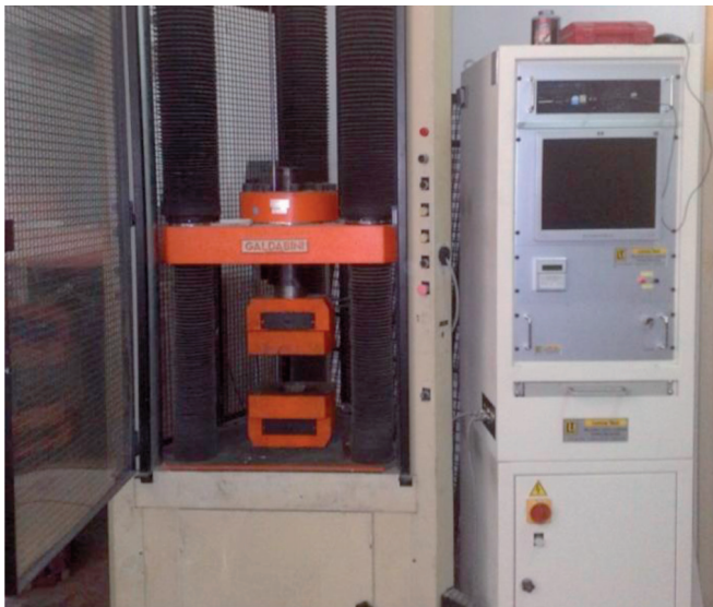
Fig. 1. Galdabini traction/compressive test machine
