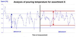
Fig. 1. Various positions of upper and lower specification limits of pouring temperature tolerance in the automatic moulding line, implemented by a "branch specialist" for the same assortment, for two different time periods as a consequence of manufacturing technology change for the assortment X
