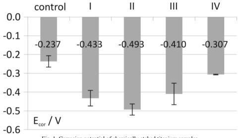
Fig. 1. Corrosion potential of chemically etched titanium samples
