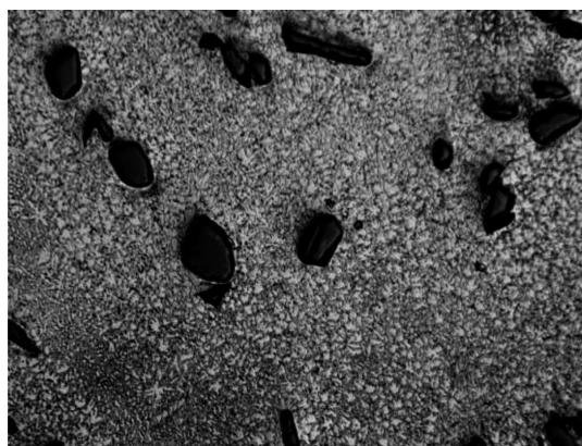
Fig. 13. Central zone of the AZ61 alloyed with SiC particles, scan rate: 0.75 m/min, laser power: 2.0 kW, mag. 500x
