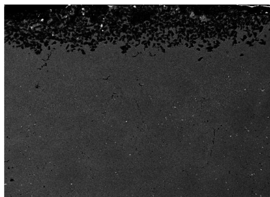
Fig. 15. Surface layer of the AZ61 alloyed with SiC particles, scan rate: 0.75 m/min, laser power: 1.6 kW, mag. 100x
