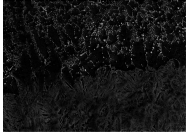
Fig. 8. 32CrMoV12-28 steel alloyed with TiC powder, SE SEM, mag. 1000x
