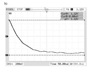
Fig. 3. Experimental characteristics: a) fragments of signal realizations  $x(i\Delta t_p)$  from sampling intervals  $\Delta t_p$  equal subsequently to:  $\Delta t_{p1} = 50 \, \mu s$ ,  $\Delta t_{p2} = 100 \, \mu s$ , and  $\Delta t_{p3} = 200 \, \mu s$ ; b) function of the conditional mean value of the analyzed signal  $\bar{x}_w = f(k\Delta t_{p1})$ .
