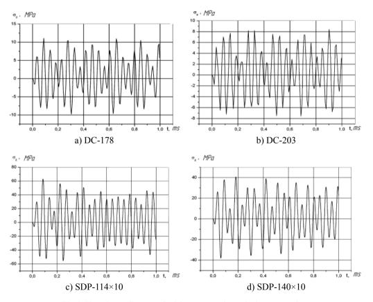
Fig. 3. Time change diagrams of axial stress  $\sigma_z$  on the stuck pipe outer surface
