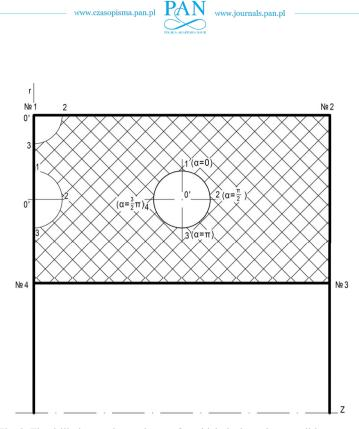
Fig. 2. The drill pipe section under test for which the boundary conditions are set
