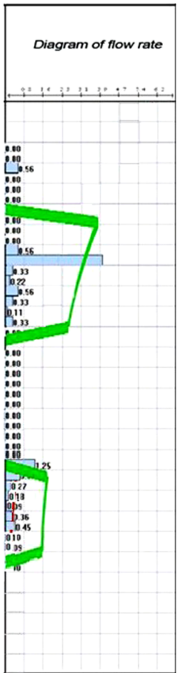
Fig. 9. Qualitative comparison of the calculation results with the data from the industrial experiment. The green curve shows the flow rate q(z) at multi-stage setting filters for the problem (13)
