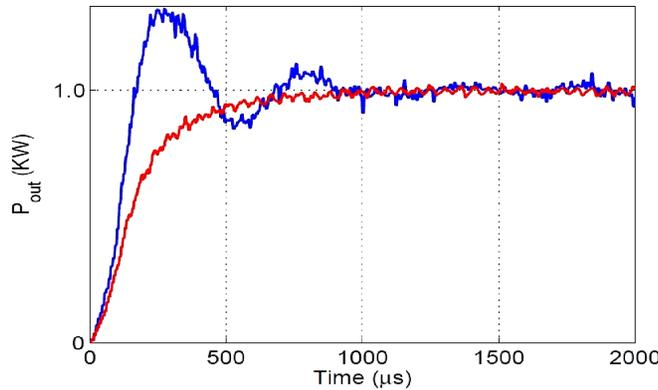
Figure 8: Comparison of power regulation for PID (blue) and robust (red) control systems with 40% variation in primary and pickup tuning inductances  $L_T$  and  $L_{si}$
