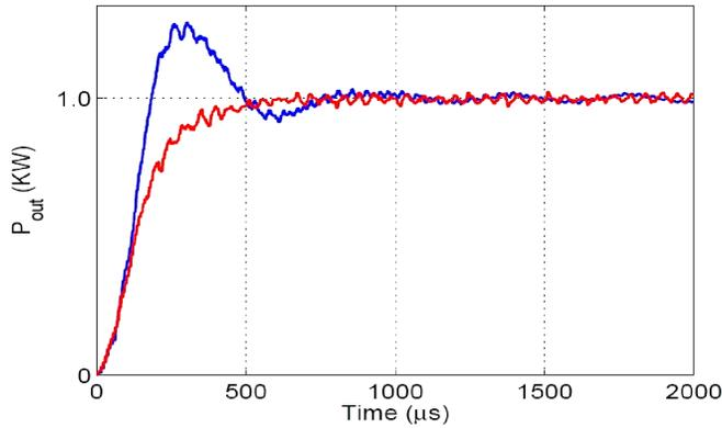
Figure 7: Comparison of power regulation for PID (blue) and robust (red) control systems with 40% variation in primary tuning capacitance  $C_T$
