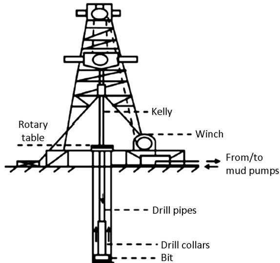
Figure 1: Drilling system
