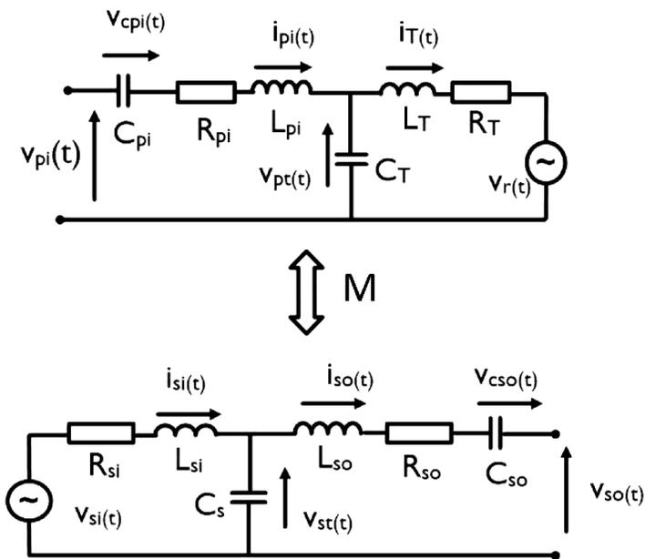
Figure 2: Equivalent circuit of a bidirectional system
