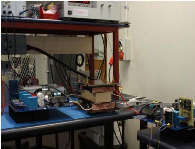
Figure 9: Prototype Bidirectional IPT system used for verification
