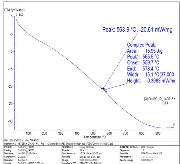
Fig. 5. DTA of 90% Silica-10% Kaolin Mixture
