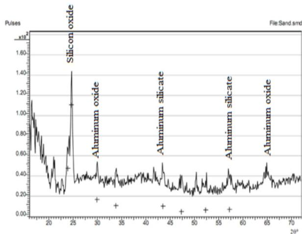
Fig. 8. X-ray diffraction of the Silica Sand
