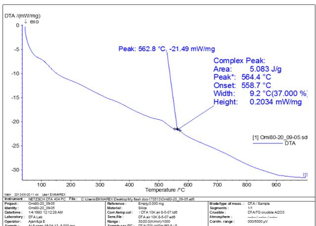
Fig. 7. DTA of 80% Silica-20% Kaolin Mixture
