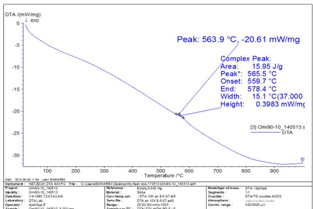
Fig. 6. DTA of 85% Silica-15% Kaolin Mixture
