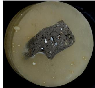
Fig. 2h. Results of the copper droplets coagulation after the R2, R3, St1, St2, St3 (5% of each), and St4 (2%) - chemical treatment performed for 20 minutes
