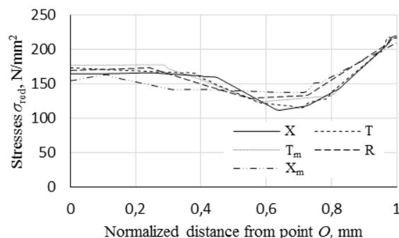
Fig. 12. Distribution of reduced stresses in the direction OC after 0.5s
