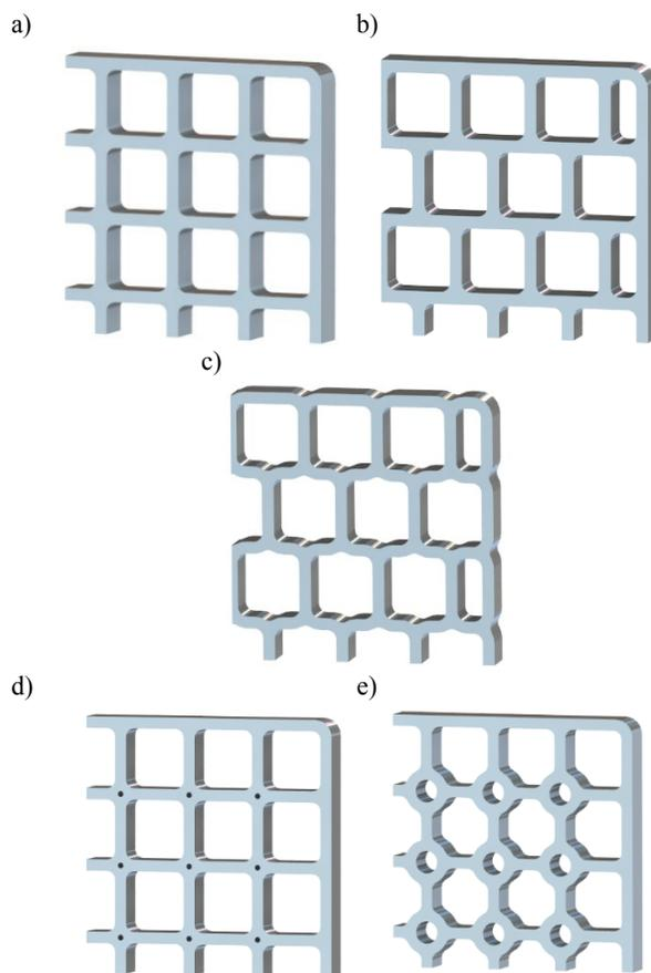
Fig. 2. Models of grate design with different types of connections adopted in the analysis: a) **X**, b) **T**, c) **T<sub>m</sub>**, d) **X<sub>m</sub>**, e) **R**
