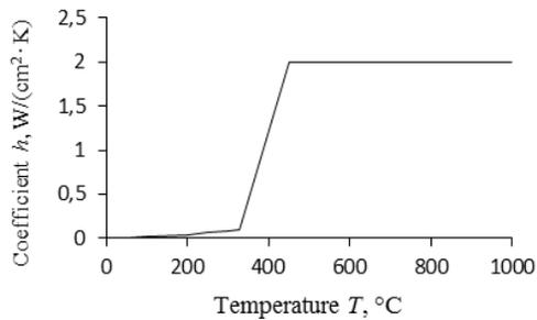
Fig. 3. Coefficient of heat transfer during cooling
