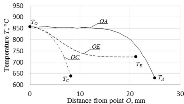
Fig. 10. Temperature distribution in the  $X$ -type connection in the directions  $OA$ ,  $OC$  and  $OE$  after 1.5s of the cooling process
