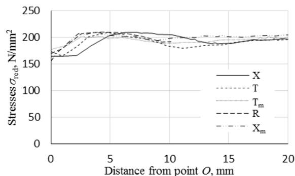
Fig. 11. Distribution of reduced stresses in the direction OE after 0.5s
