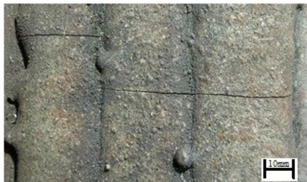
Fig. 11. Cracks in the wide bead
