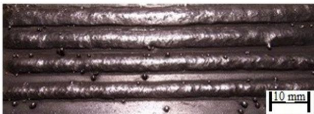
Fig. 6. Spatter on the surface
