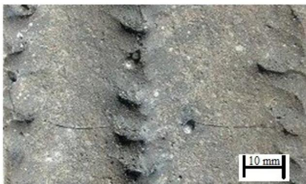
Fig. 16. Face inequalities by automatic welding.
