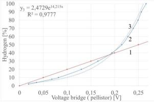
Fig. 3. Variants of the calibration of the pellistor bridge voltage:
