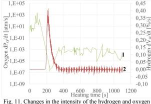
Fig. 11. Changes in the intensity of the hydrogen and oxygen emission: 1 - oxygen, 2 – hydrogen
