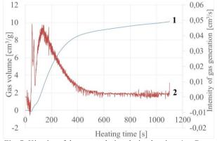
Fig. 7. Kinetics of the gas evolution during heating: 1 – Gases emission from the moulding sand, 2 – Gases evolution rates (kinetics)
