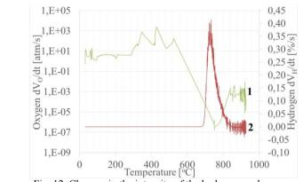
Fig. 12. Changes in the intensity of the hydrogen and oxygen emission in relation to a temperature: 1 - oxygen, 2 - hydrogen
