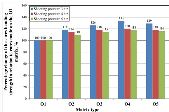
Fig. 8. Percentage change of the cores bending strength in relation to cores made on the O1 matrix
