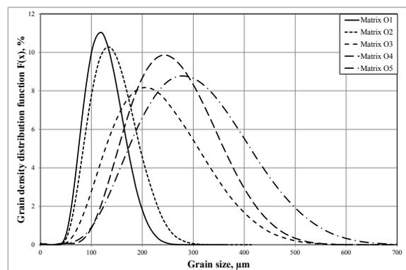
Fig. 3. Grain density distribution function  $F(x)$  for matrices O1÷O5
