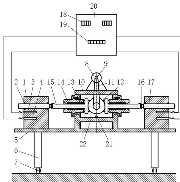
Fig.1 Experimental apparatus of valve body wearing
