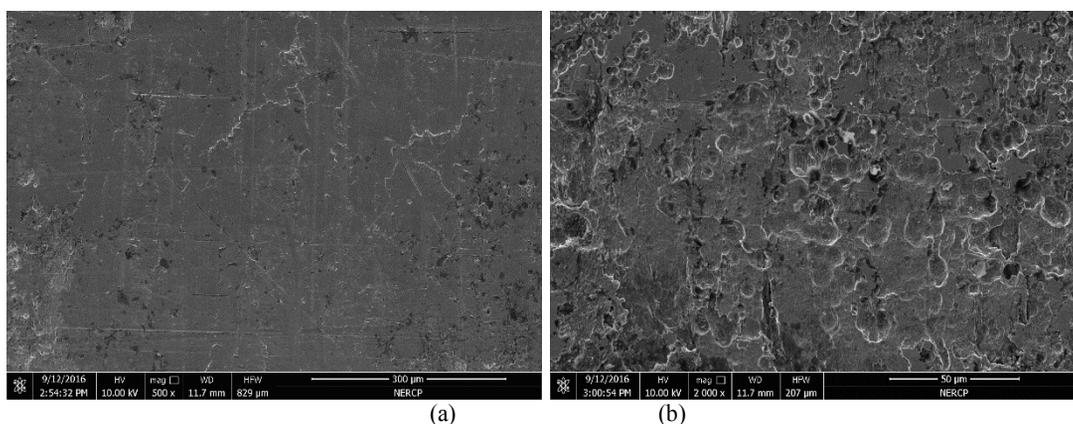
Fig. 6. Cast iron valve after 600,000 cycles' times
