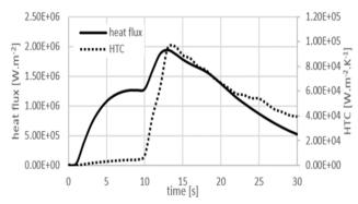
Fig. 2. Heat flux and HTC between the cast and the mold at the temperature of casting 690 °C, pressure 100 MPa
