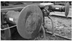
Fig. 1. Railway buffers mounted on headstock of freight car
