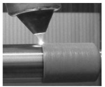
Fig. 3. A view of laser powder cladding process of the rod made of steel S355J2 by aluminum bronze using a high power diode laser HPDL
