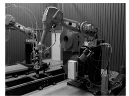
Fig. 2. A view of the robotic stand equipped with a high power diode laser HPDL LDF 4000-30 LaserLine
