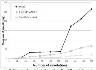
Fig. 9. The mass loss of tested samples after 200 revolutions, at the normal force 700 N
