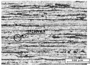
Fig. 4. Microstructure of S355J2 steel in the delivery condition; Mag. 200x; Etching- Nital, longitudinal microsection
