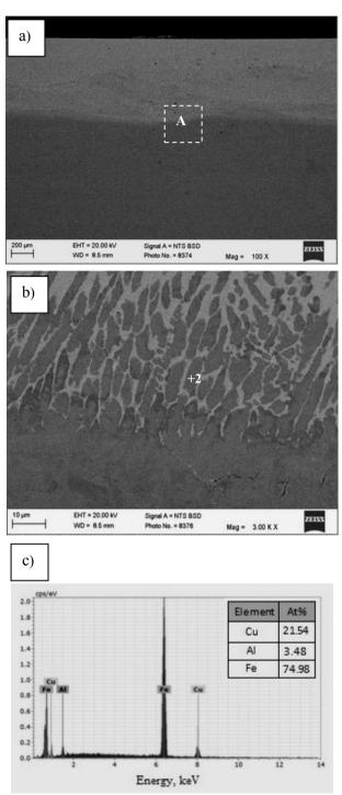
Fig. 6. Microstructure of the single layer clad of CuAl9Fe3 bronze on the substrate of S355J2 steel produced by laser cladding (a), transverse section unetched; b) detail "A" from the Fig. a microstructure of CuAl9Fe3 bronze, under SEM examination;
