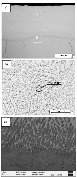
Fig. 5. Cross-section of the single layer clad of CuAl9Fe3 bronze on the substrate of S355J2 steel produced by laser cladding (a), transverse section unetched, Mag. 100x; b) detail "A" from the Fig. a - microstructure of CuAl9Fe3 bronze, etched longitudinal section, Mag. 200x; c) detail "B" from the Fig. a - fusion line under SEM examination
