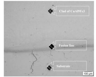
Fig. 7. Cross-section of the single layer clad of aluminum bronze CuAl9Fe3 on the steel substrate with marked points of hardness measurements
